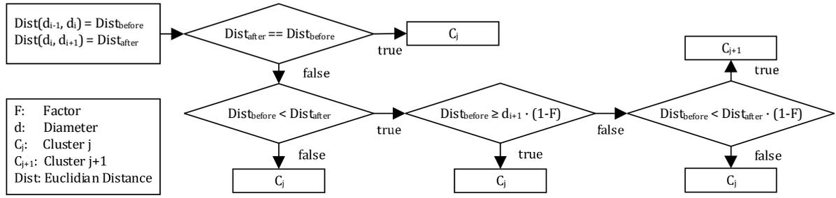
Fig. 3. Linked Parts Clustering Algorithm.
