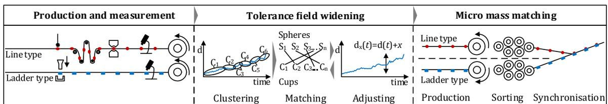
Fig. 1. Concept of mass matching of micro parts.
